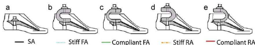
Fig. 1. Ankle conditions: (a) solid ankle, SA, (b) stiff forward-facing ankle, FA, (c) compliant FA, (d) stiff reverse-facing ankle, RA, and (e) compliant RA. The pylon attached directly to the Seattle Lightfoot2 for the SA condition, whereas the ankle was attached between the pylon and the Seattle Lightfoot2 for the other four ankle conditions.
